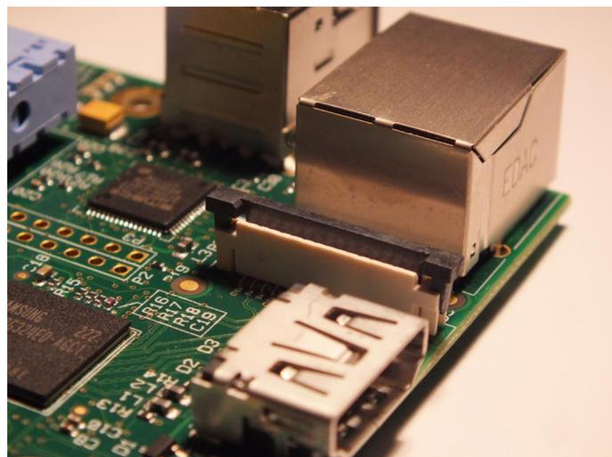
It should slide up easily, and be able to pivot around slightly. Fully insert the ribbon cable into the slot, ensuring it is straight, then gently press down the tabs to clip it into place. The camera PCB itself also requires you to pull the tabs away from the board, gently insert the cable, then push the tabs back.
