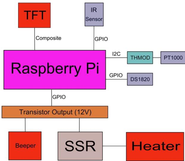
To use a Raspberry Pi as a brewing controller, two main interfaces had to be added. The first
