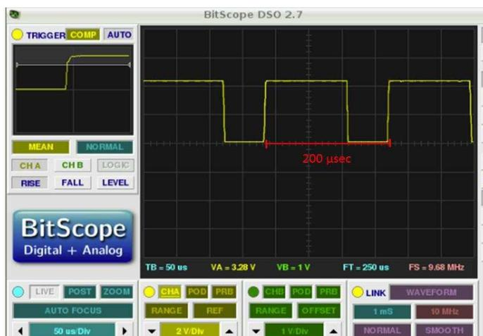
**Fig. 8:** Output of the clock generator circuit
