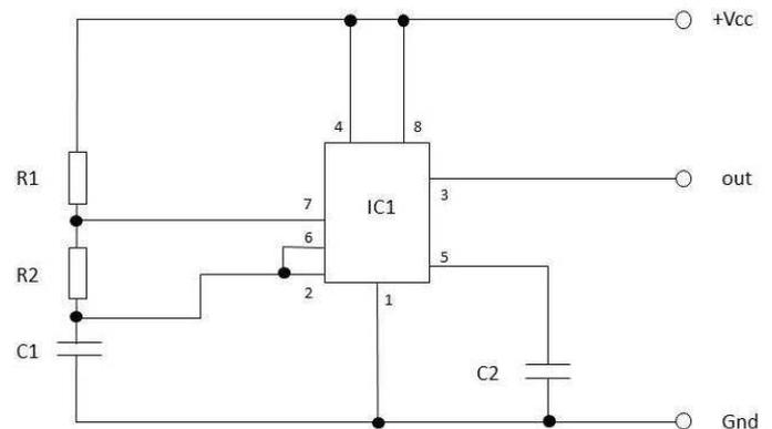
**Fig. 5:** Circuit diagram of the clock generator
