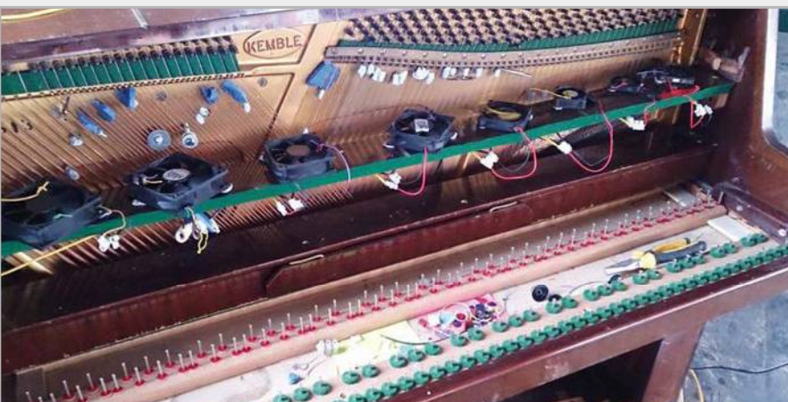
Noisy Toys hooked hardware to piano strings and processed the sounds through analogue synth boards for intriguing new tones
