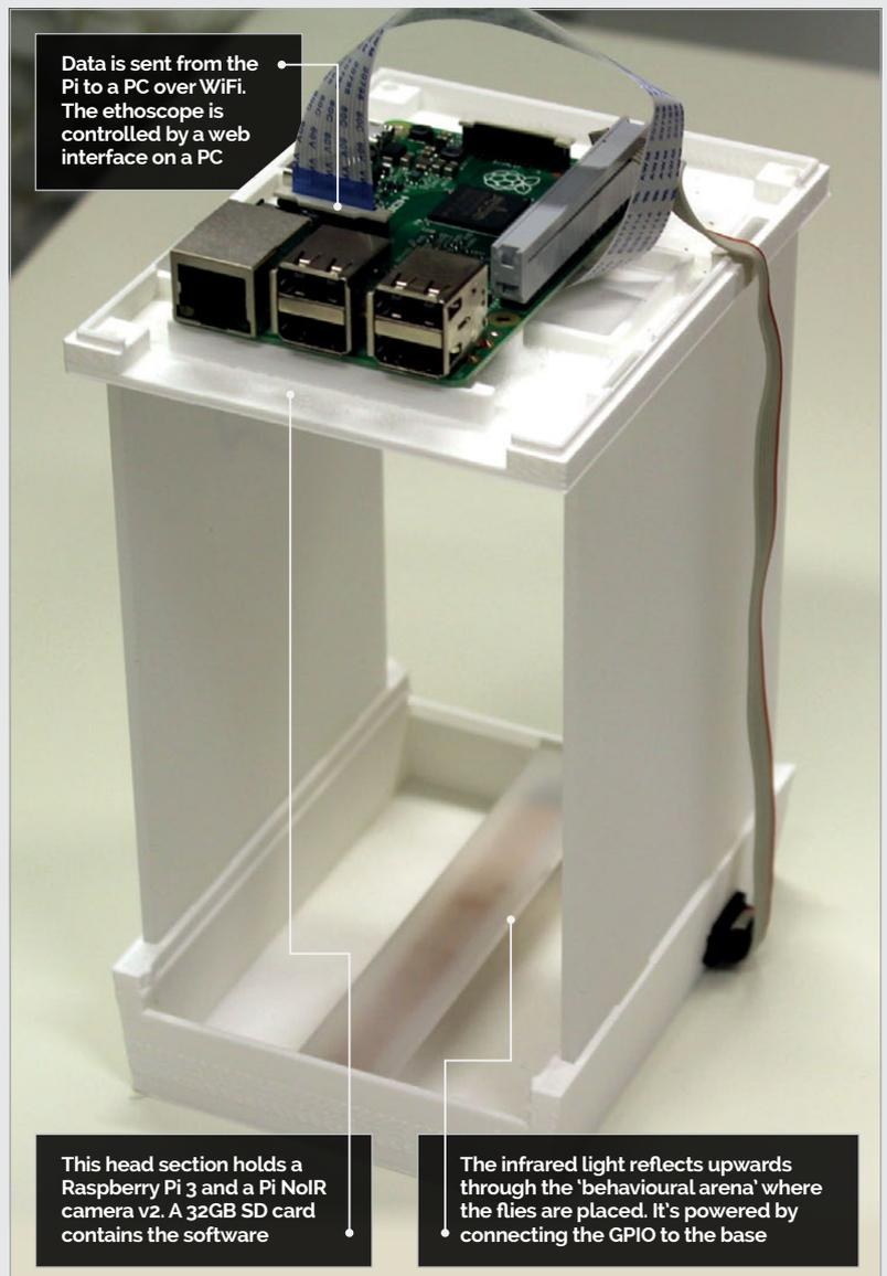
maybe thousands of flies at once because [the ethoscopes] are so small and cheap to maintain,” explains Giorgio. “By using the Pis, we have enough computer power to analyse their behaviour using video
