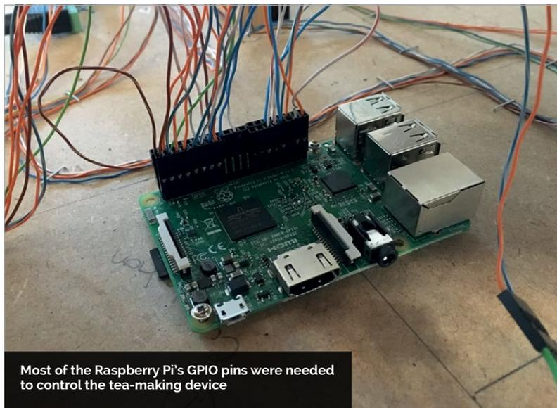
Most of the Raspberry Pi’s GPIO pins were needed to control the tea-making device
