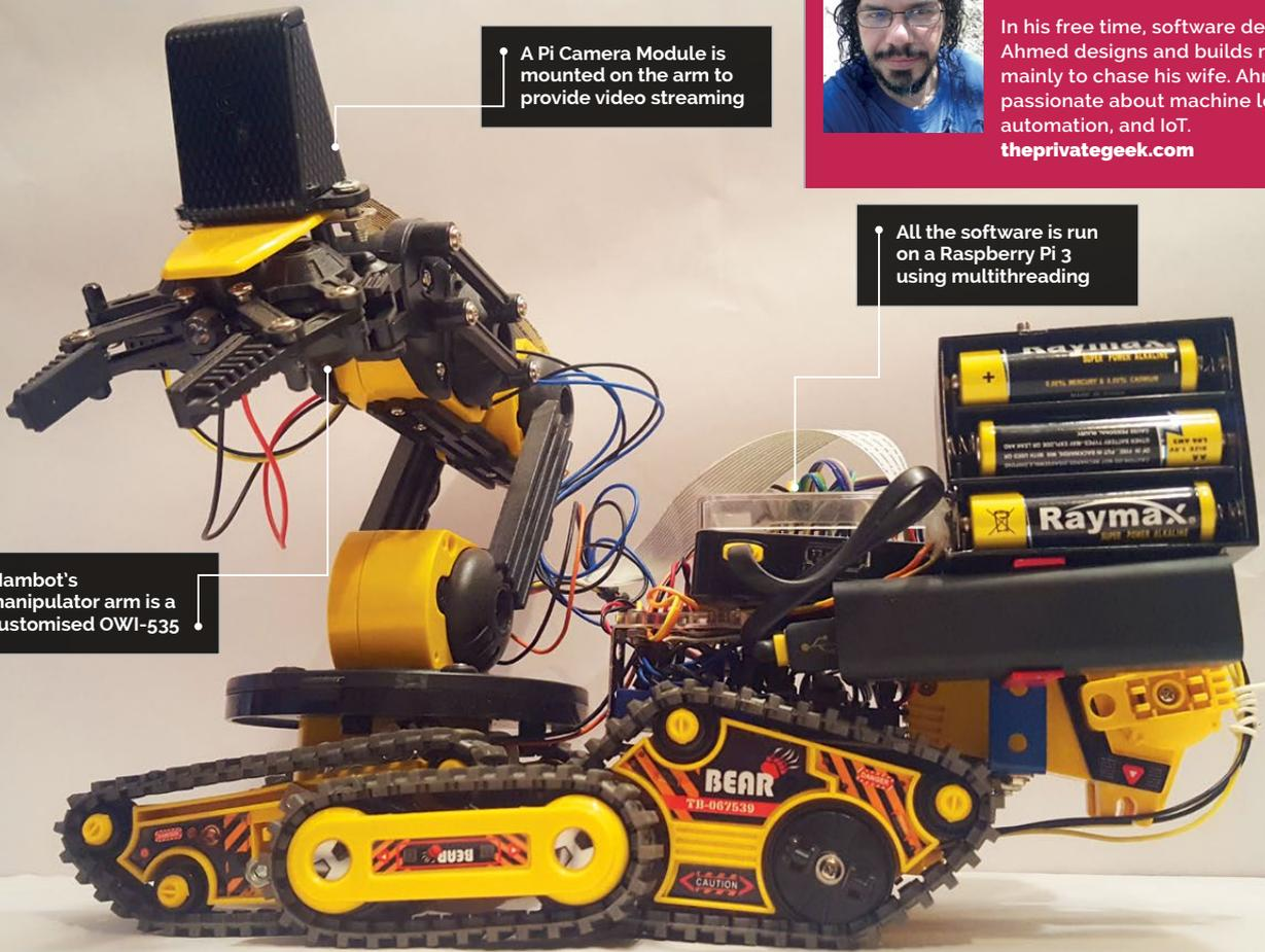
A Pi Camera Module is mounted on the arm to provide video streaming
