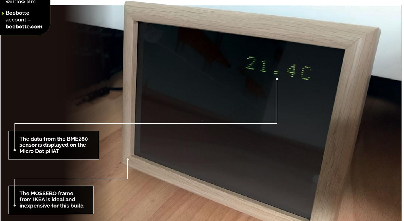
The data from the BME280 sensor is displayed on the Micro Dot pHAT
