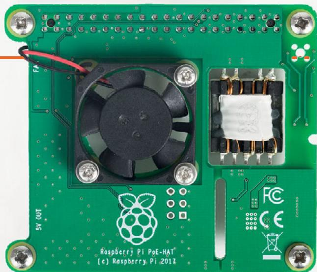
Because the 3B+ is the only Raspberry Pi to feature these additional PoE pins, you must use this HAT with a Raspberry Pi 3B+ (no other model is currently supported).
