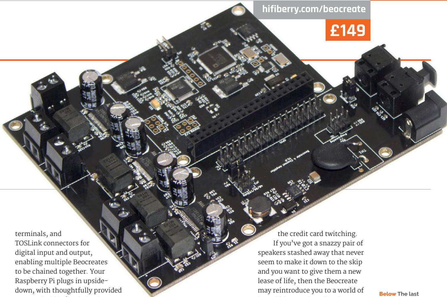
terminals, and TOSLink connectors for digital input and output, enabling multiple Beocreates to be chained together. Your Raspberry Pi plugs in upside-down, with thoughtfully provided posts to hold it firmly in place. You can then power both boards from a single power supply (not supplied).
