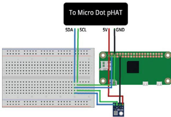
Above The BME280 is connected to 3V, GND, SDA, and SCL pins on the Pi. The Micro Dot pHAT is connected to 5V, GND, SDA, and SCL as well
