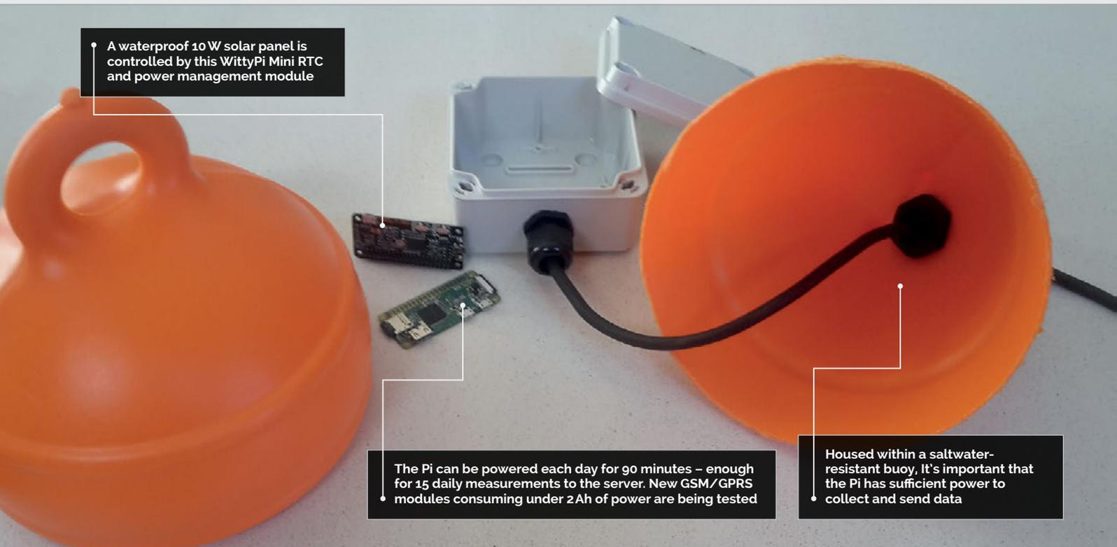
A waterproof 10 W solar panel is controlled by this WittyPi Mini RTC and power management module
