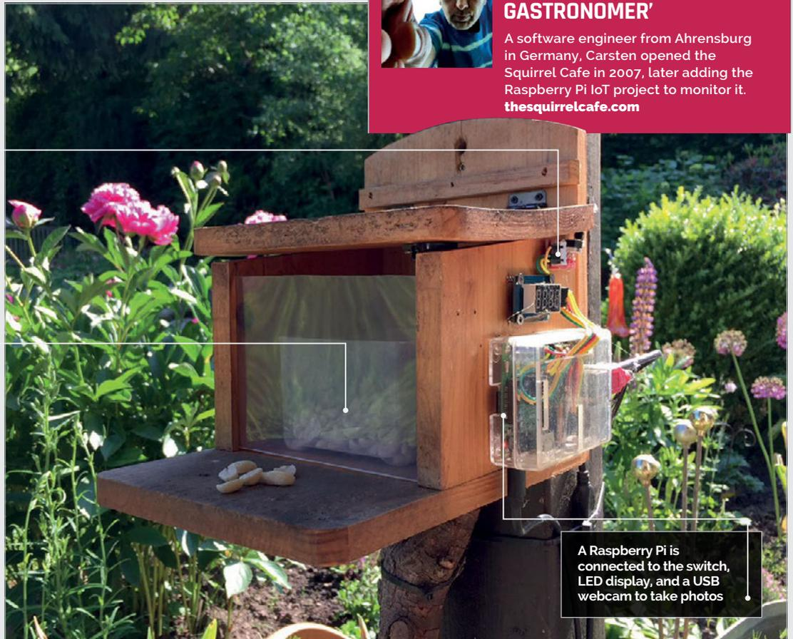
A Raspberry Pi is connected to the switch, LED display, and a USB webcam to take photos
