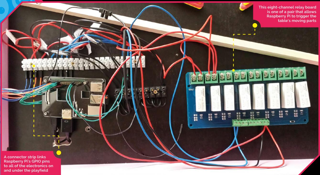
This eight-channel relay board is one of a pair that allows Raspberry Pi to trigger the table's moving parts
