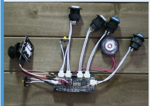
02 The analogue thumb joystick, six buttons, and 0.25W 8Ω speaker were connected to an Adafruit Arcade Bonnet. A couple of freely available scripts were then run to get everything working.
