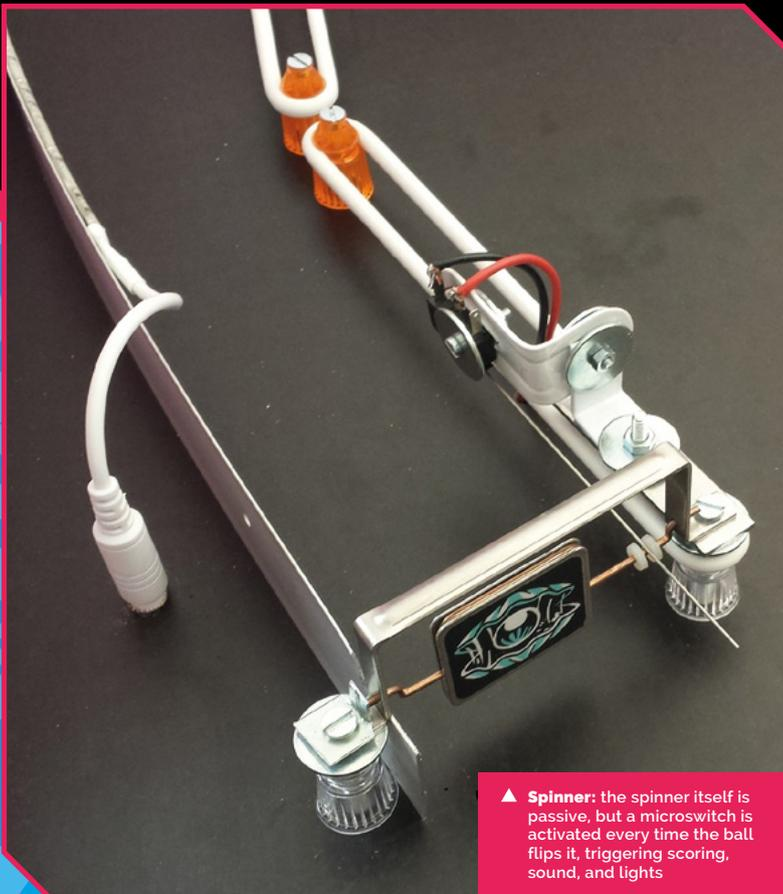
▲ **Spinner:** the spinner itself is passive, but a microswitch is activated every time the ball flips it, triggering scoring, sound, and lights
