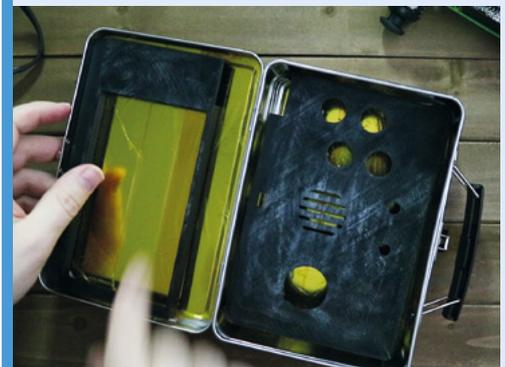
03 After careful measuring, Daniel designed and 3D-printed a screen holder, which he hot-glued to the lunchbox lid, and a board to house the arcade controls and speaker.
