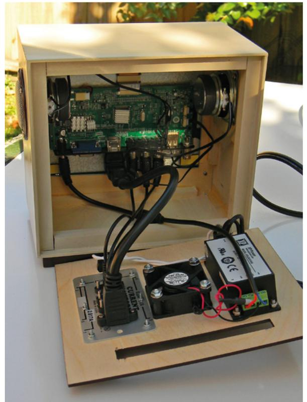
▶ Cables run from the circuit board of the monitor to the back of the new case, so that the connectors are easily accessible. Components are cooled by a fan
