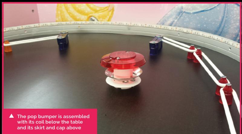
▲ The pop bumper is assembled with its coil below the table and its skirt and cap above
