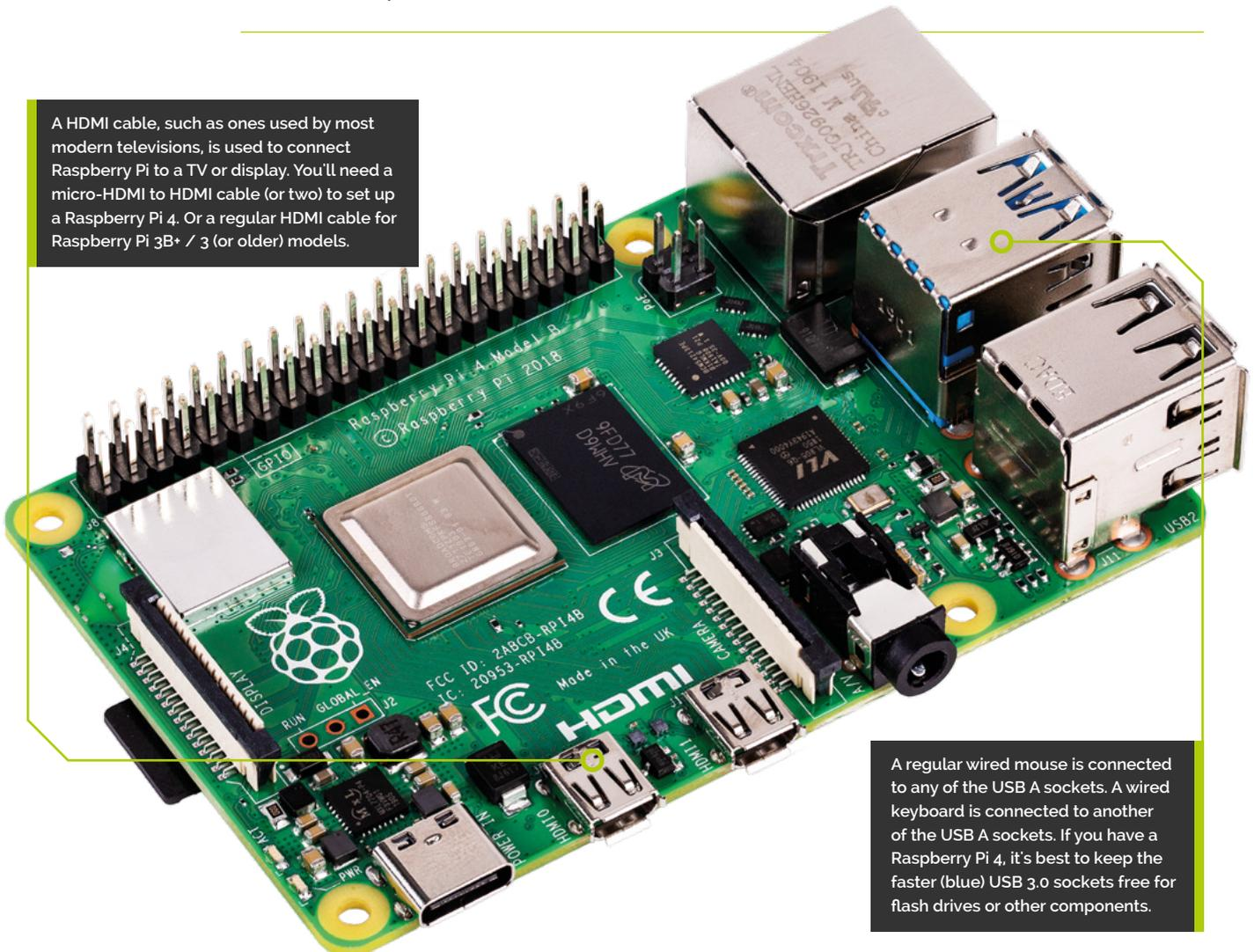
A regular wired mouse is connected to any of the USB A sockets. A wired keyboard is connected to another of the USB A sockets. If you have a Raspberry Pi 4, it's best to keep the faster (blue) USB 3.0 sockets free for flash drives or other components.
