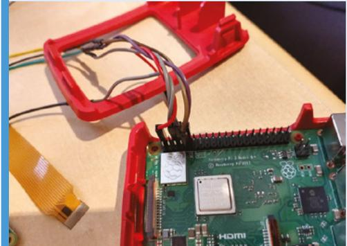
**01** A Raspberry Pi 3B+ was used to trigger the water spray, lights, and fans, bringing an extra element to the gameplay, as well as rendering the arcade machine’s graphics.
