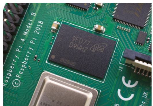
▲ Raspberry Pi 4 with 2GB and 4GB models are identical designs, bar the memory module used, and fully compatible with each other's software and accessories
