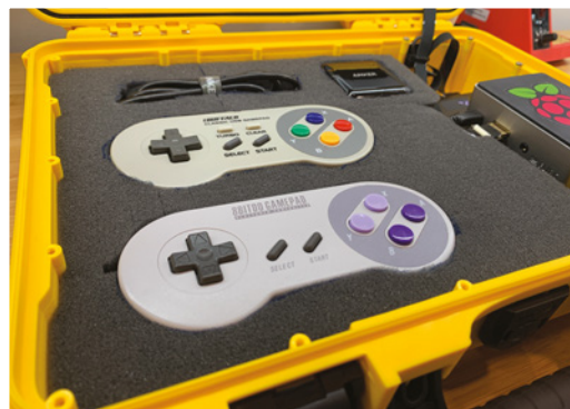
▶ The Console Edition is essentially a Raspberry Pi with RetroPie installed connected to a display in a case with foam inserts for controllers and accessories
