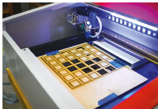
▲ Alex eventually got a laser cutter to help speed up production – like for these mounting grids
