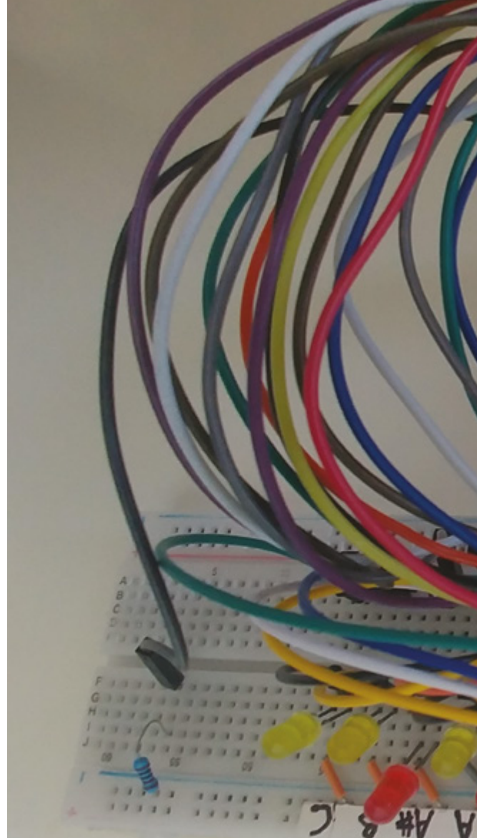
▲ To test the setup away from the bell tower, a piano layout of LEDs was created, each LED representing a note / bell
