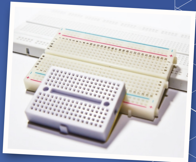
▲ Breadboards come in several sizes to enable prototyping of a wide variety of projects
