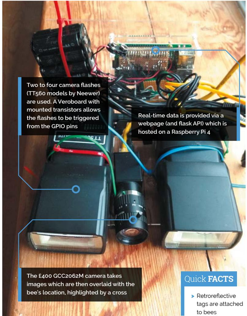
Two to four camera flashes (TT560 models by Neewer) are used. A Veroboard with mounted transistors allows the flashes to be triggered from the GPIO pins
