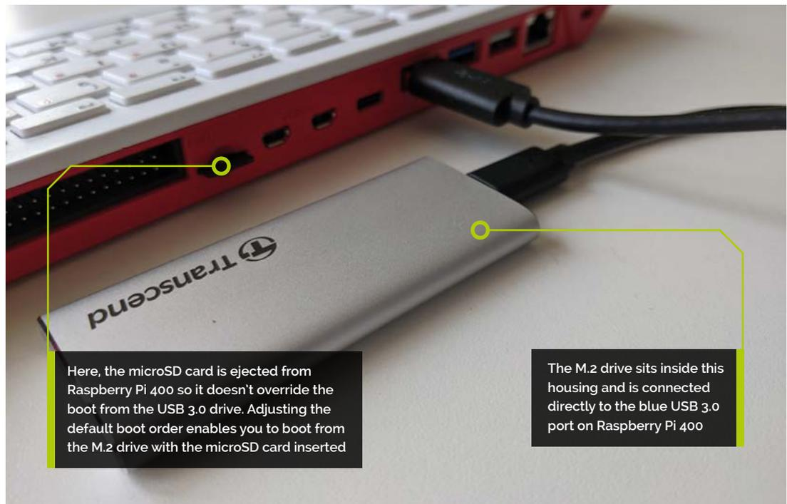
Here, the microSD card is ejected from Raspberry Pi 400 so it doesn't override the boot from the USB 3.0 drive. Adjusting the default boot order enables you to boot from the M.2 drive with the microSD card inserted
