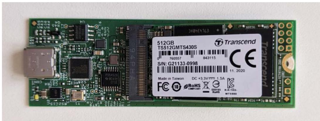
◀ The M.2 SSD adapter translates the SATA III interface on the M.2 SSD drive into a USB-C connection. This is used with a USB-C to USB-A cable to connect the drive to the blue USB 3.0 connection on Raspberry Pi 400
