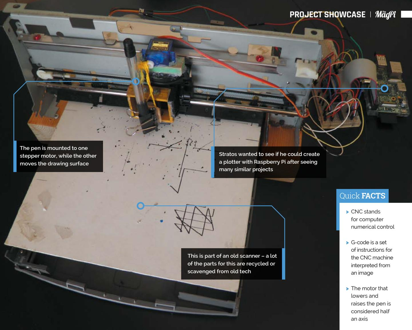
The pen is mounted to one stepper motor, while the other moves the drawing surface
