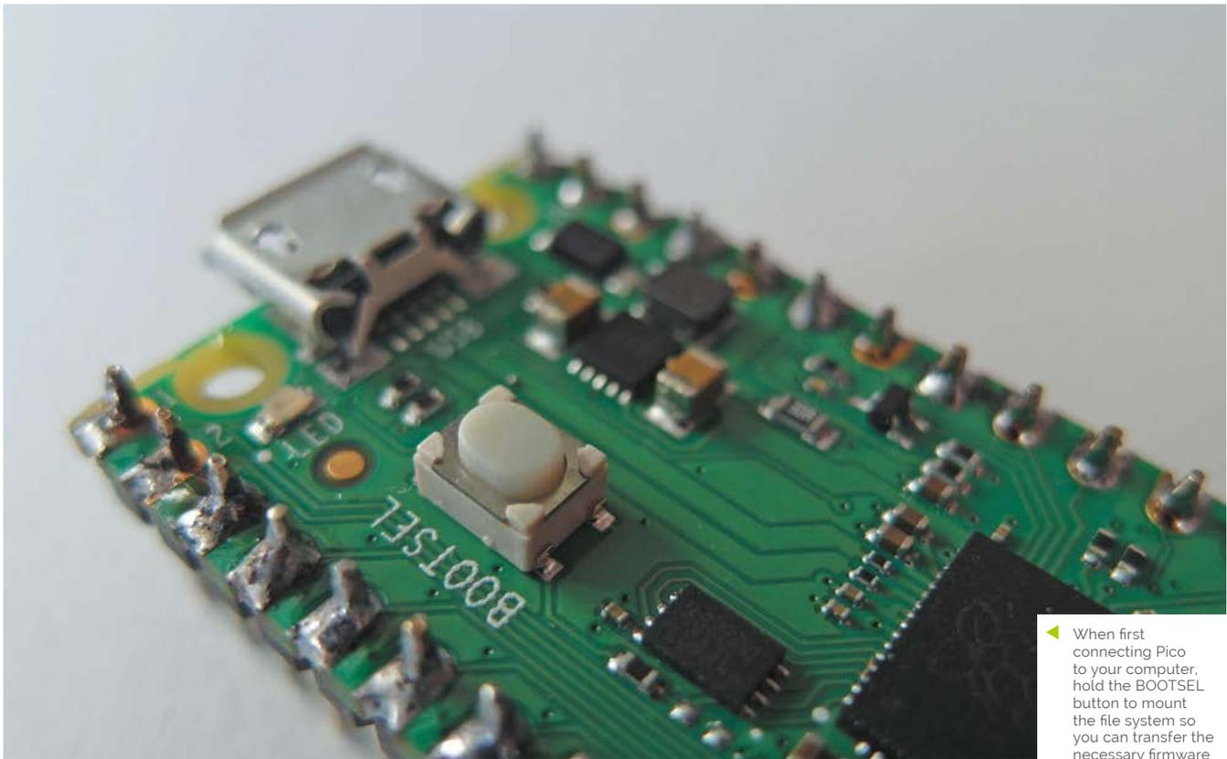
◀ When first connecting Pico to your computer, hold the BOOTSEL button to mount the file system so you can transfer the necessary firmware
