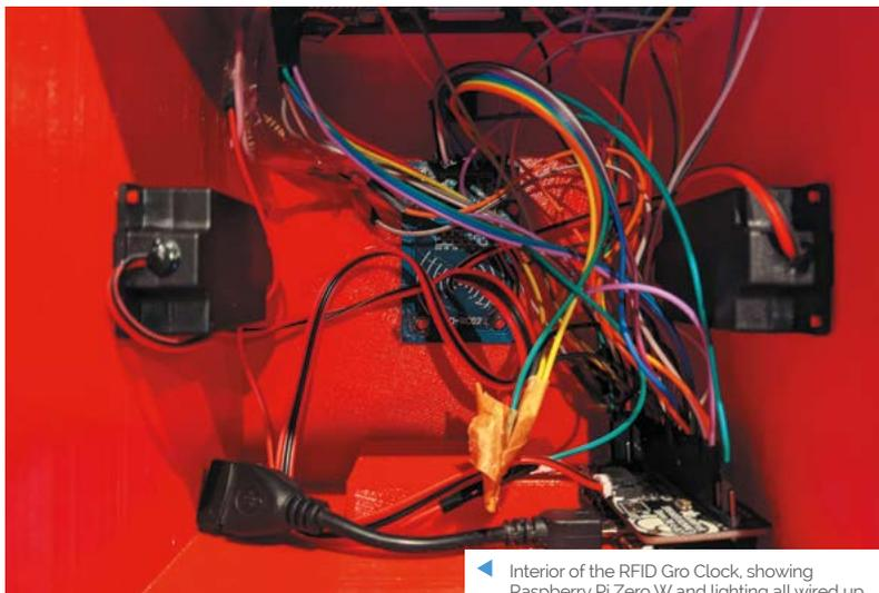
Interior of the RFID Gro Clock, showing Raspberry Pi Zero W and lighting all wired up
