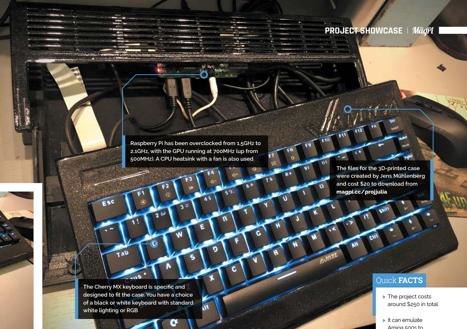
Raspberry Pi has been overclocked from 1.5GHz to 2.1GHz, with the GPU running at 700MHz (up from 500MHz). A CPU heatsink with a fan is also used
