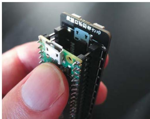
◀ When fitting the Unicorn Pack to Pico, match the rear illustration to the USB socket to make sure it's correctly orientated
