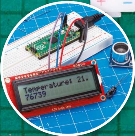
Electronic components, like the SparkFun SerLCD display and sensors pictured can be tested out in the breadboard, and then wired up directly to Pico
