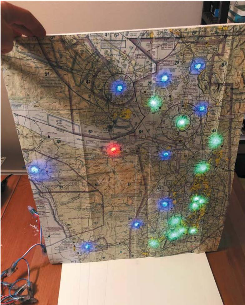
Refinements include making the lights blink if there are high winds at an airport, and another addition to make the LEDs flash white if there is a lightning storm in the area. He's recently added a small LCD which shows full weather information for the airports.
