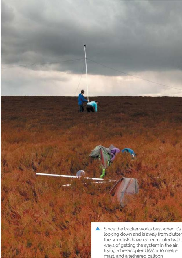
▲ Since the tracker works best when it's looking down and is away from clutter, the scientists have experimented with ways of getting the system in the air, trying a hexacopter UAV, a 10 metre mast, and a tethered balloon
