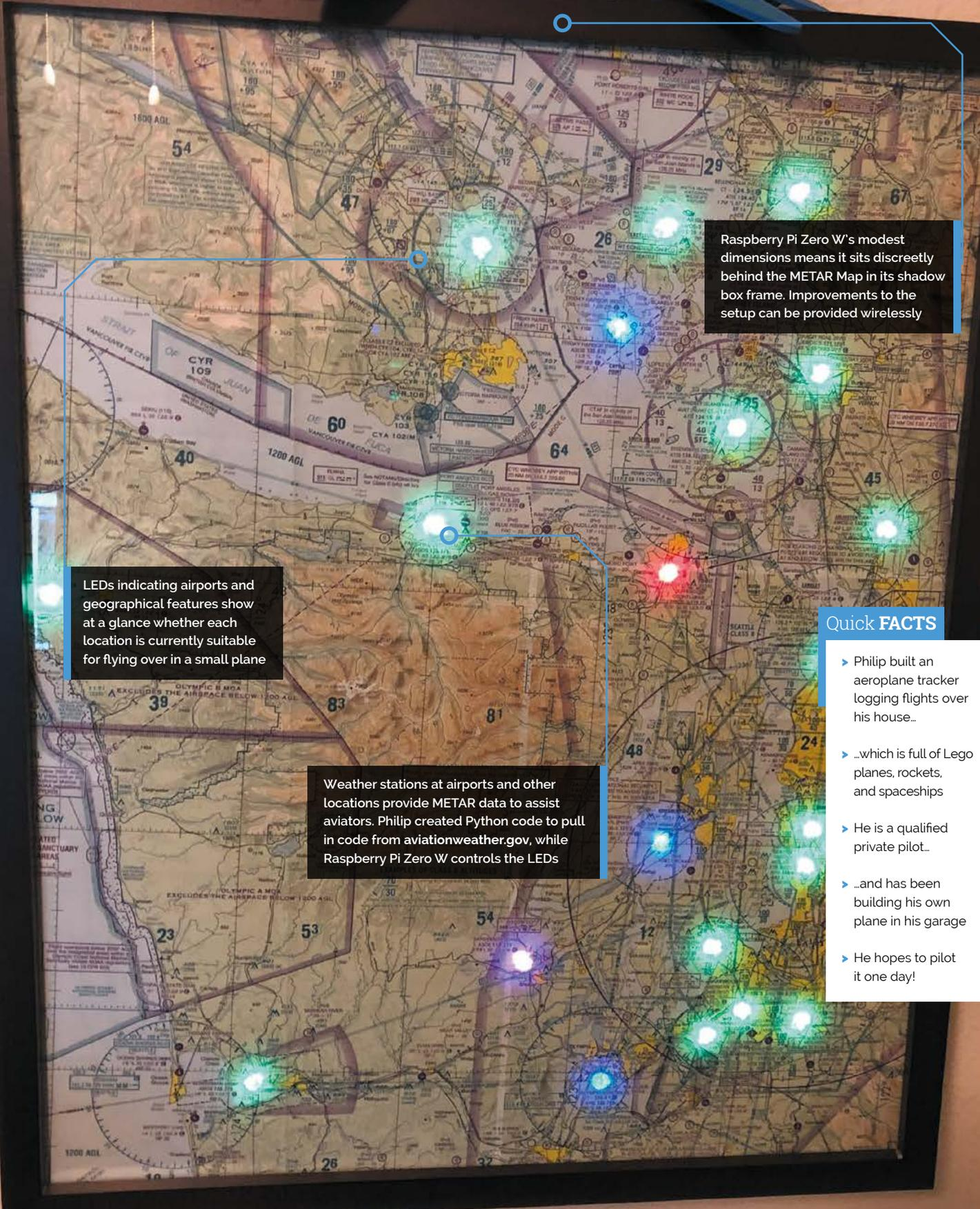
Raspberry Pi Zero W's modest dimensions means it sits discreetly behind the METAR Map in its shadow box frame. Improvements to the setup can be provided wirelessly
