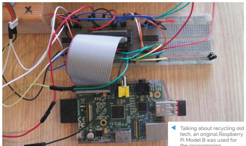
◀ Talking about recycling old tech, an original Raspberry Pi Model B was used for the programming
