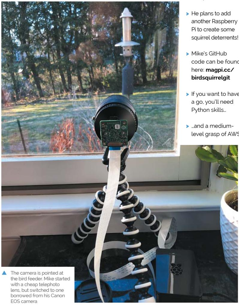
▲ The camera is pointed at the bird feeder. Mike started with a cheap telephoto lens, but switched to one borrowed from his Canon EOS camera
