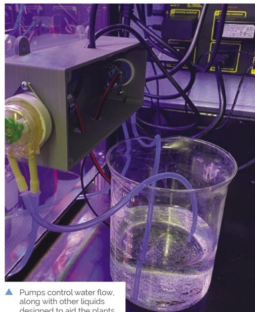
▲ Pumps control water flow, along with other liquids designed to aid the plants
