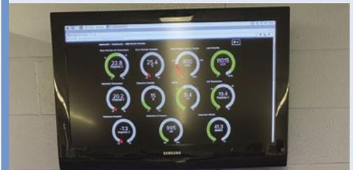
**03** “All data is viewable in real time and historically, while all actuators are controllable via our Adafruit IO dashboard. Adjustment parameters like RGBW light spectrum, photoperiod, fan speed, pH and temperature set points, and liquid dosing volumes can be chosen here as well.”
