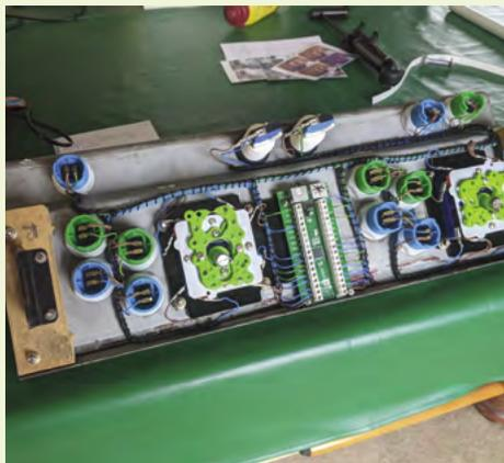
“ There's room to slide the screw slots on most joystick mounting plates ”
