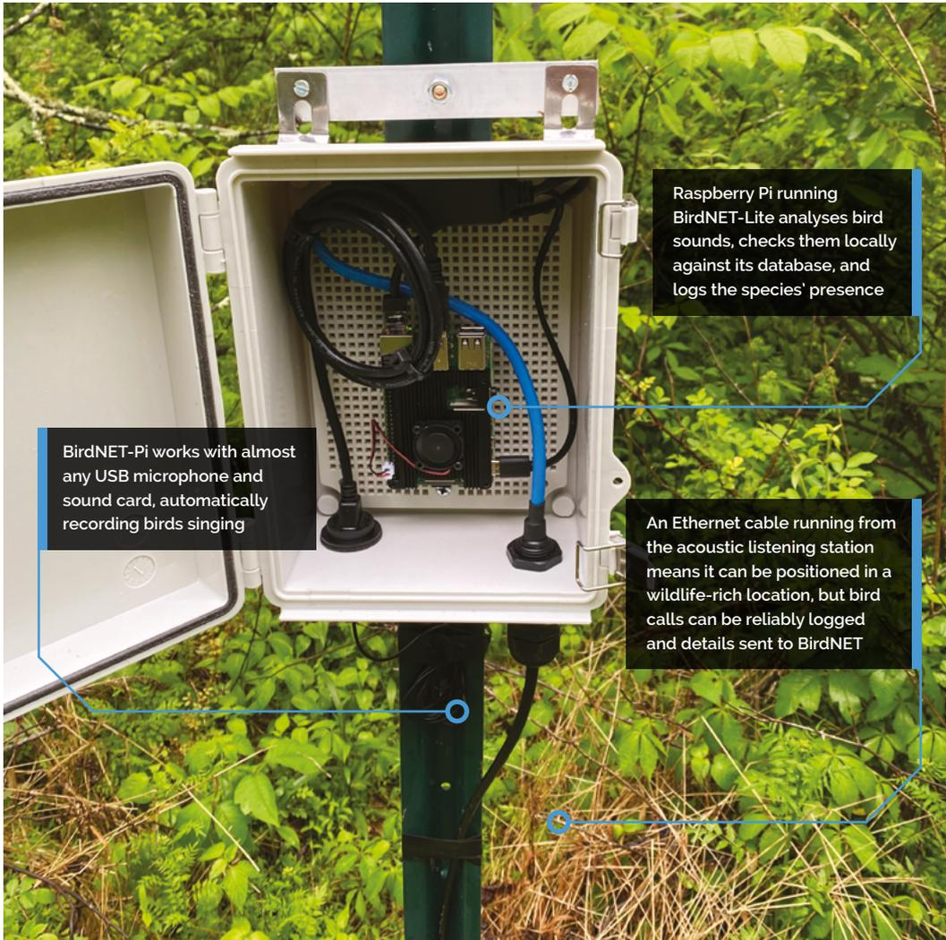
BirdNET-Pi works with almost any USB microphone and sound card, automatically recording birds singing
