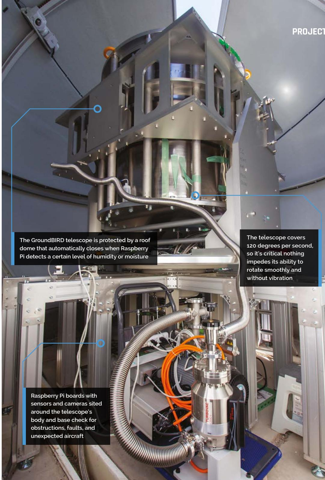
The GroundBIRD telescope is protected by a roof dome that automatically closes when Raspberry Pi detects a certain level of humidity or moisture
