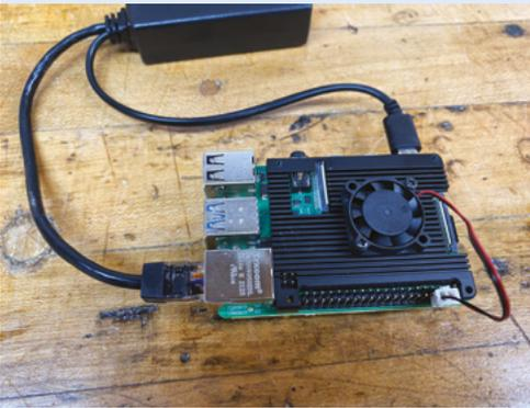
**02** The Power over Ethernet card and PoE adapter, plus a power supply with fan, ensure BirdNET-Pi can be used to remotely record and identify bird species.
