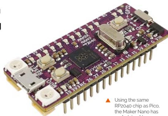
▲ Using the same RP2040 chip as Pico, the Maker Nano has an Arduino Nano-style pinout
