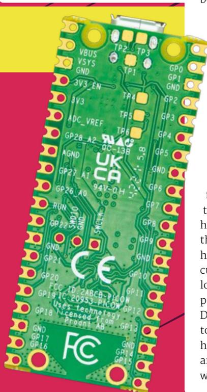
► Thanks to the clever design, all 40 GPIO pins remain in the same position on the newly designed Pico W board
