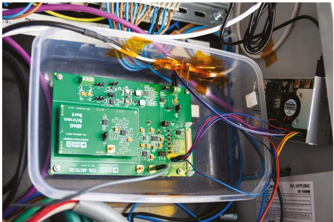
▶ The Raspberry Pi, yuzu-pi controlling the azimuth rotation through a DAC board
