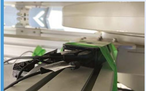
**03** Additional Raspberry Pi sensors and cameras trained on the telescope's wheels and exterior provide an early warning of faults or vibrations beyond the delicate tolerance levels.
