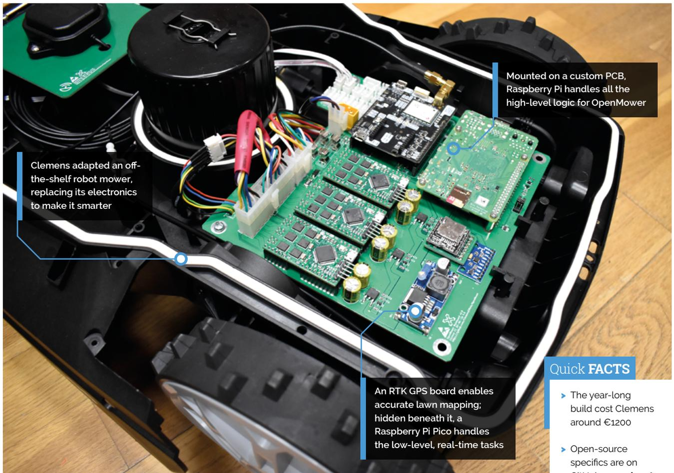
Clemens adapted an off-the-shelf robot mower, replacing its electronics to make it smarter
