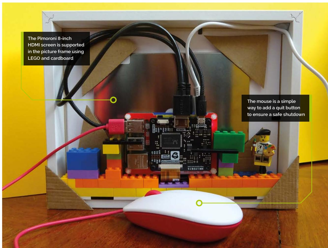
The Pimoroni 8-inch HDMI screen is supported in the picture frame using LEGO and cardboard
