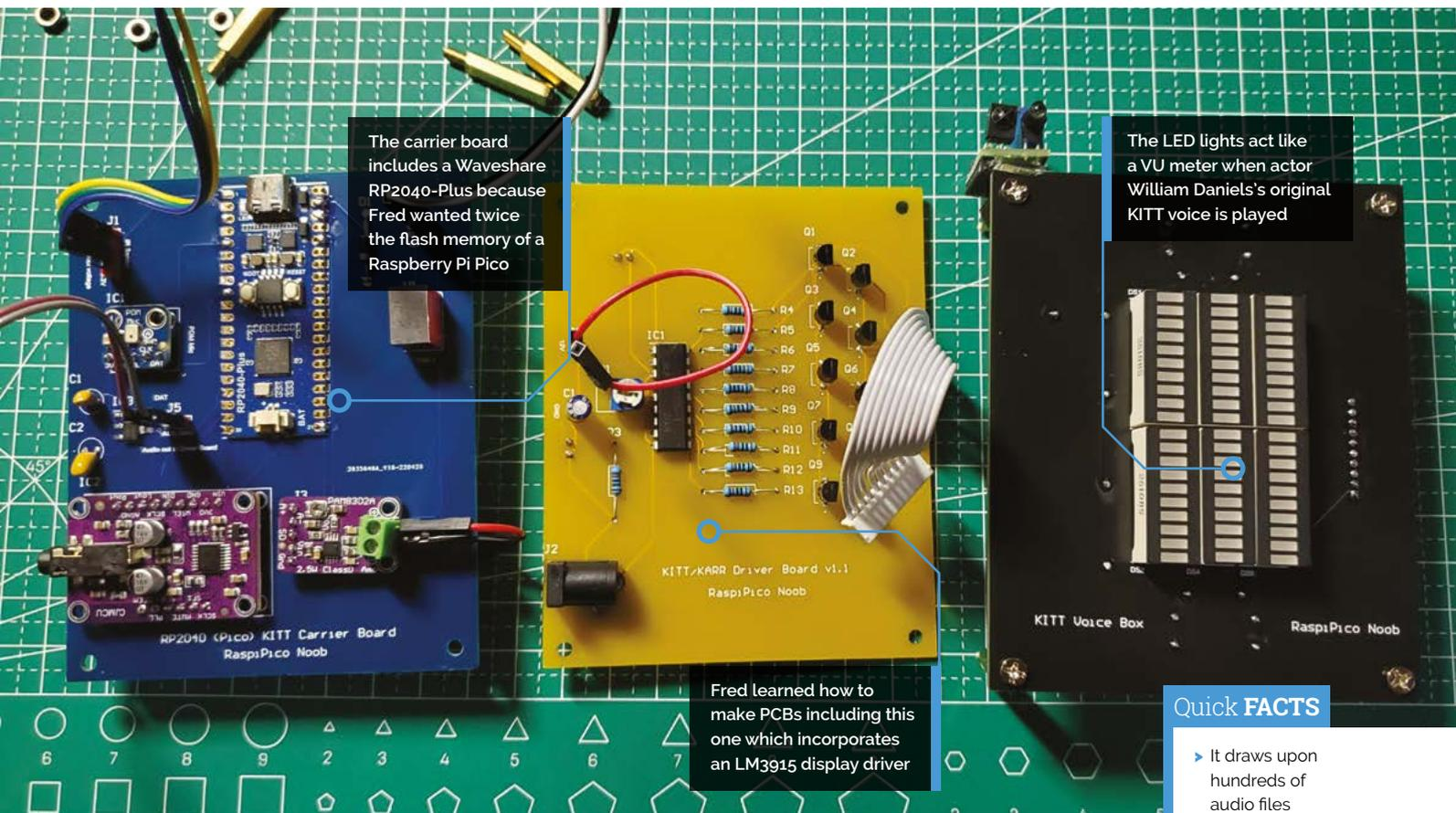
The carrier board includes a Waveshare RP2040-Plus because Fred wanted twice the flash memory of a Raspberry Pi Pico
