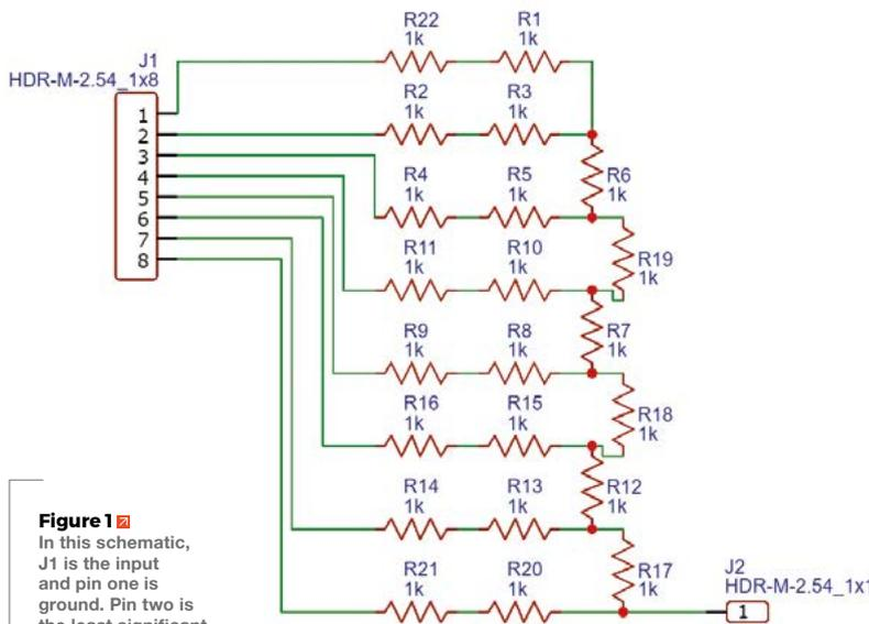
**Figure 1** In this schematic, J1 is the input and pin one is ground. Pin two is the least significant bit, and it goes up from there
