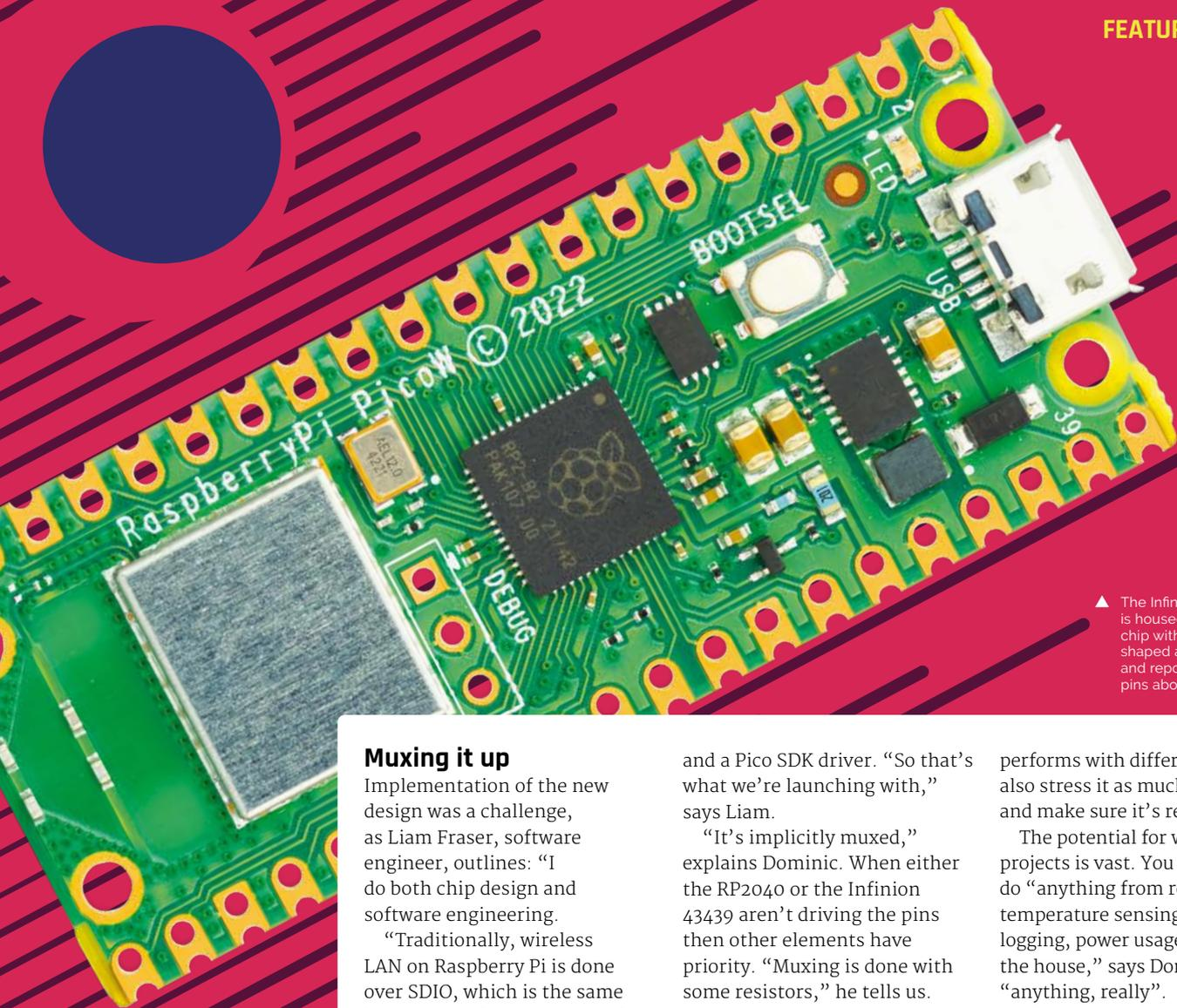
▲ The Infineon CYW4339 is housed in an enclosure chip with the trapezoid-shaped antenna below and repositioned DEBUG pins above
