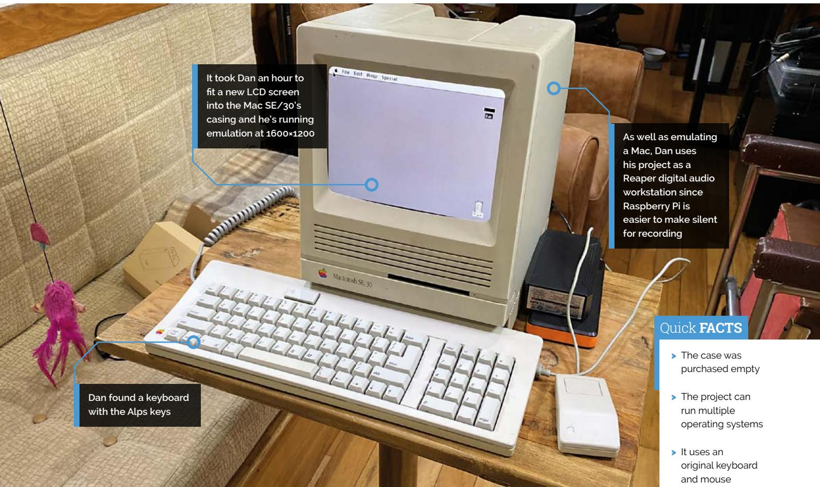
It took Dan an hour to fit a new LCD screen into the Mac SE/30's casing and he's running emulation at 1600x1200
