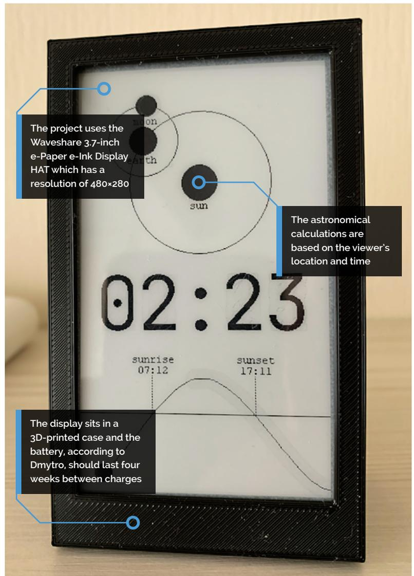
The project uses the Waveshare 3.7-inch e-Paper e-Ink Display HAT which has a resolution of 480x280
