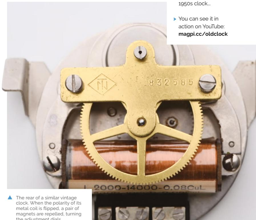
▲ The rear of a similar vintage clock. When the polarity of its metal coil is flipped, a pair of magnets are repelled, turning the adjustment dials
