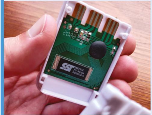
**01** The substitute memory card provides a physical interface between the Pico and the PlayStation. Access the electronic board by removing the two screws on the bottom, and take off the plastic shell. Cut a hole in the case for the wires.
