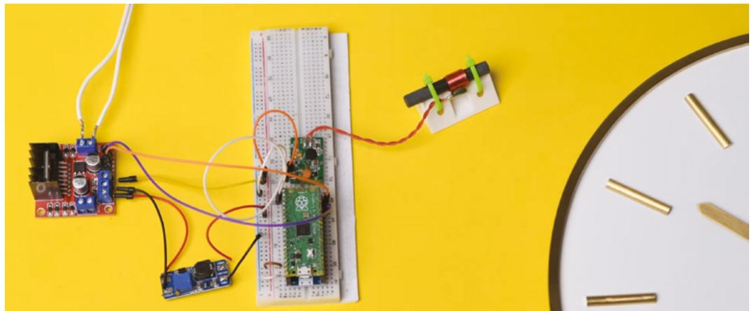
▶ Wiring up the circuit. Components include an H-bridge, step-up module, and radio antenna
