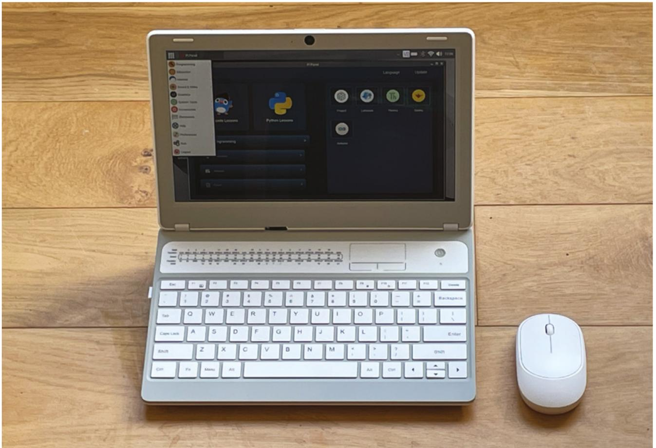
displayed a resolution of 1920×1080 with the stock Raspberry Pi OS, and a look back at config.txt in CrowPi L OS revealed custom timings to set the resolution to 1912×1079.
