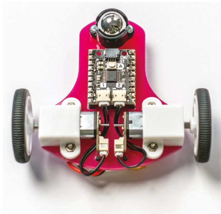
▲ The Motor SHIM fitted to the base of a simple two-wheeled robot
