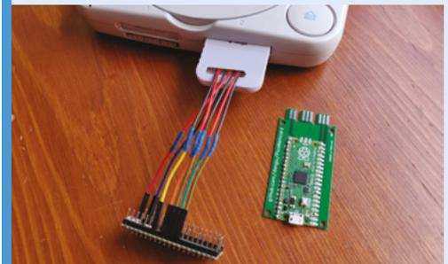
**03** Carefully solder your Pico to the PCB, download the latest version of PicoMemcard ([magpi.cc/picomemcardreleases](http://magpi.cc/picomemcardreleases)), plug your device into the computer via USB, and upload the save file.
