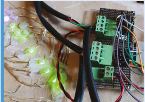
**02** The dashboard reads the API to set the NeoPixels: “The demultiplexer is needed to drive the four strings off of a single pin (pin 18). This was necessary as they are fixed-address NeoPixels. The Tfl open data site has a fairly simple REST interface, which supplies statuses as well as arrival/departure information.”
