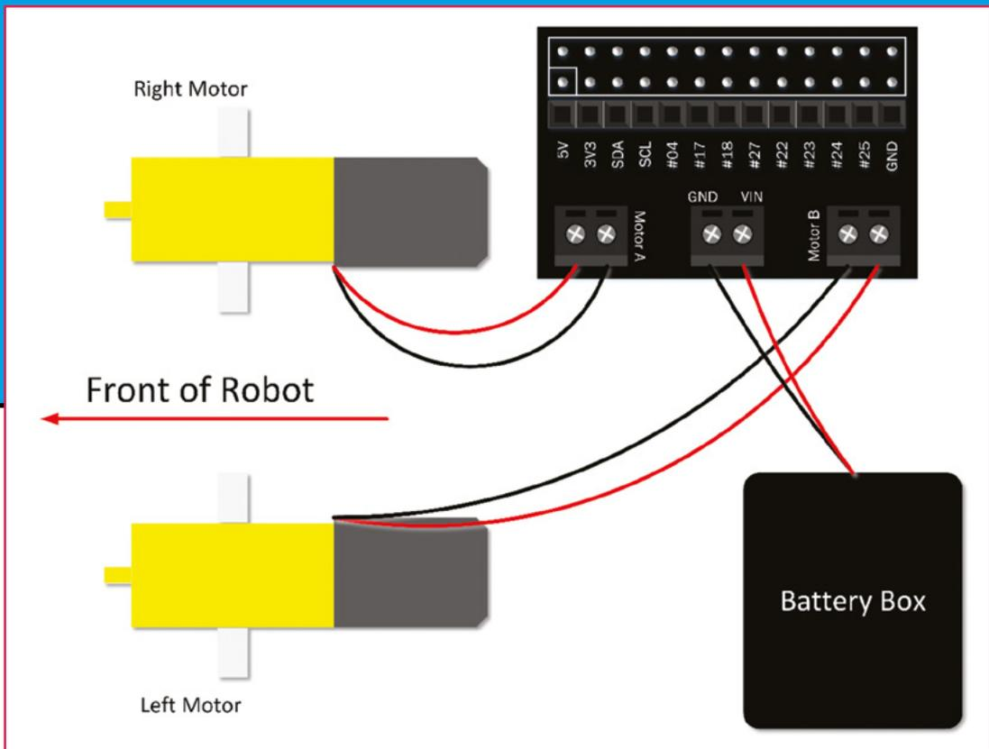
▶ Wire up the control board as shown here. This is the view looking down
