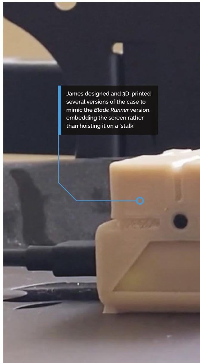
James designed and 3D-printed several versions of the case to mimic the *Blade Runner* version, embedding the screen rather than hoisting it on a 'stalk'
