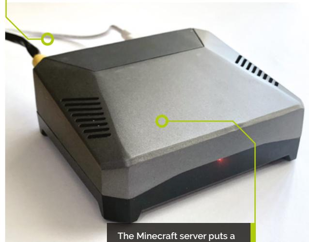
The Minecraft server puts a lot of strain on a Raspberry Pi 4B, so a good case with built-in cooling is essential
