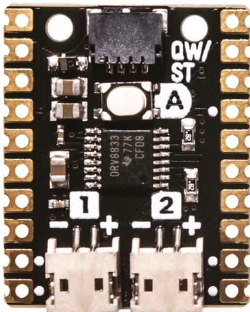
► As well as two JST-ZH motor connectors, there's an on-board push-button and Qwiic/STEMMA QT port
