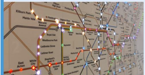
**03** The LEDs are lit up in a specific manner to represent different statuses. “It enables me to quickly know there was a problem, how long the problem lasted, and how serious it was. In one case, I was able to arrange some help to be dispatched... following a failure.”
