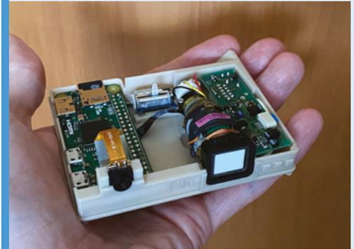
**01** To recreate the Voight-Kampff machine, you’ll need a Raspberry Pi Pico, HQ camera, a suitable enclosure, and the CRT display from a camcorder. James designed and 3D-printed a case for his.
