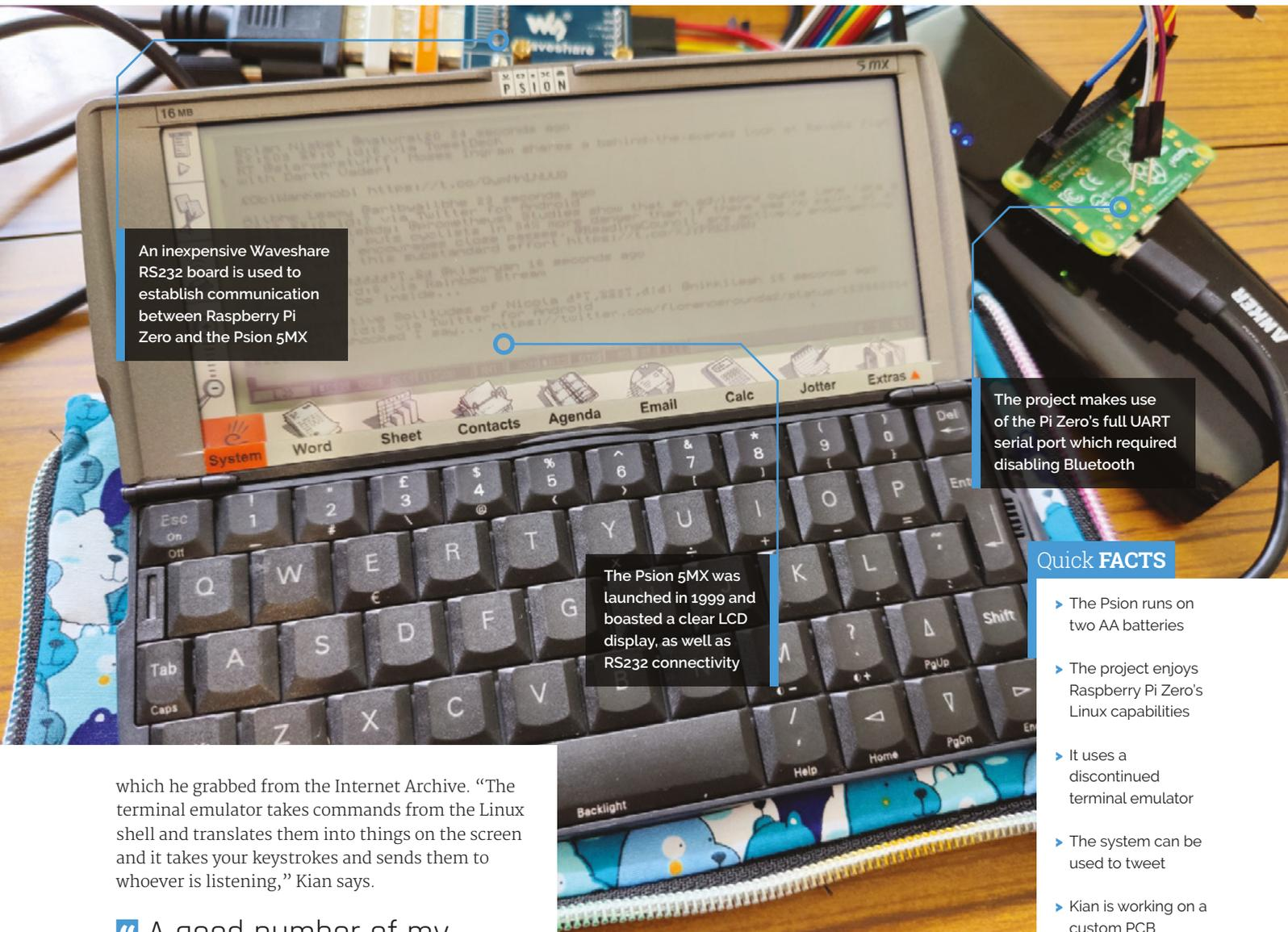
An inexpensive Waveshare RS232 board is used to establish communication between Raspberry Pi Zero and the Psion 5MX
