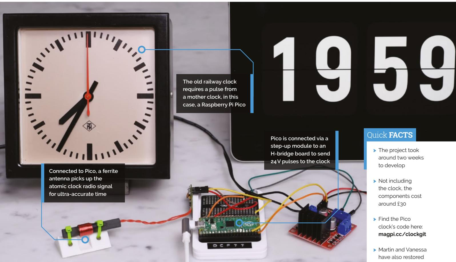
Connected to Pico, a ferrite antenna picks up the atomic clock radio signal for ultra-accurate time
