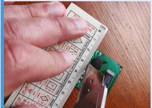
**02** Use a Stanley/utility knife to cut a groove right under the pins and disconnect the original circuitry. Use jumper wires to connect your Pico, scraping off their plastic covering, and directly soldering to the copper pins for the PlayStation.
