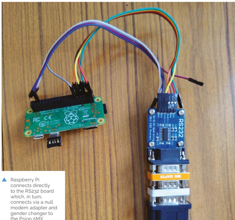
▲ Raspberry Pi connects directly to the RS232 board which, in turn, connects via a null modem adapter and gender changer to the Psion 5MX
