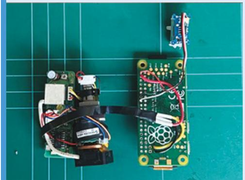
**02** A servo drives mini bellows, like those in the original film. The servo is controlled using the pigpio library directly from a GPIO pin. No extra hardware is needed.
