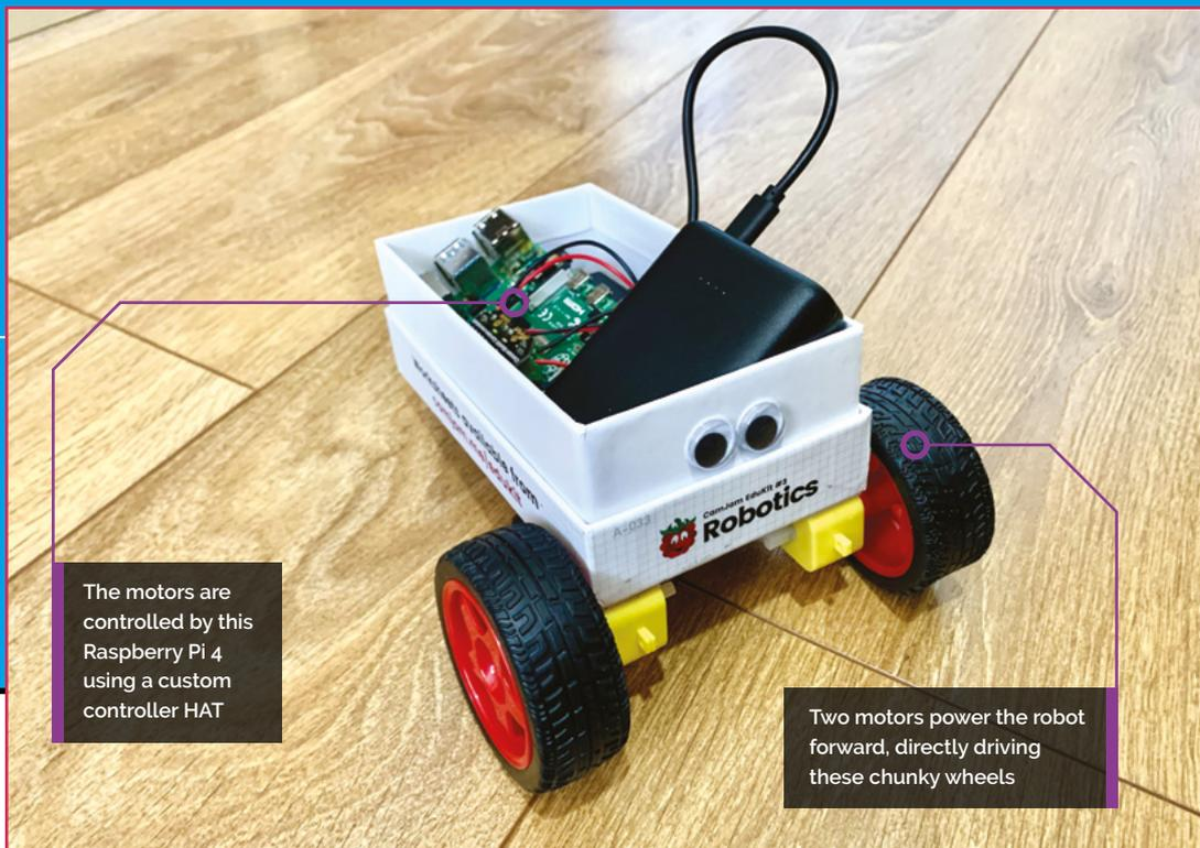
The motors are controlled by this Raspberry Pi 4 using a custom controller HAT
